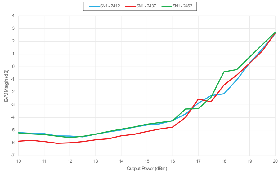
Figure 8 ■ Spectral Mask Margin versus Output Power for 2412, 2437, and 2462 MHz, MCS0 Waveform
