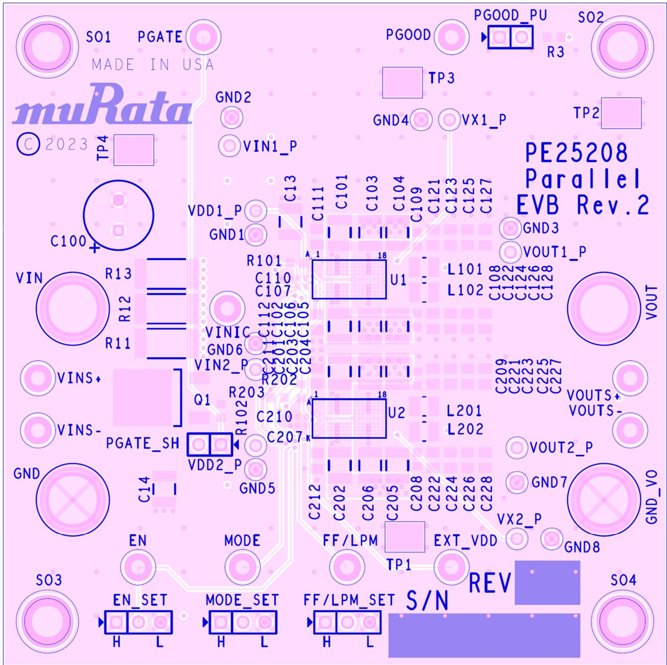
Figure 14. Inner Layer 2 (PWR and Signal) PCB Layout of the PE25208 Parallel EVK
